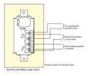
The End-of-Line Relay facilitates the connection of a non-polarized releasing solenoid to a supervised, polarized releasing circuit. One relay is required per release solenoid.
