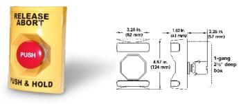
The abort station is a normally-open, non-latching device. It is used to prevent the release of agent into the protected area after the release sequence has begun.
