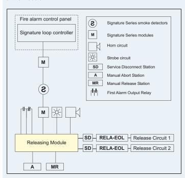
Release Circuits. The SIGA-REL includes two supervised release circuits, each of which provides fire suppression control to different areas of a protected space. The releasing circuits actuate solenoids on the suppression agent tanks according to pre-defined release routines. These solenoids release the agent into the protected area. Both circuits operate together.
