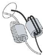
Fig 8: Safety ground and ferrite bead
