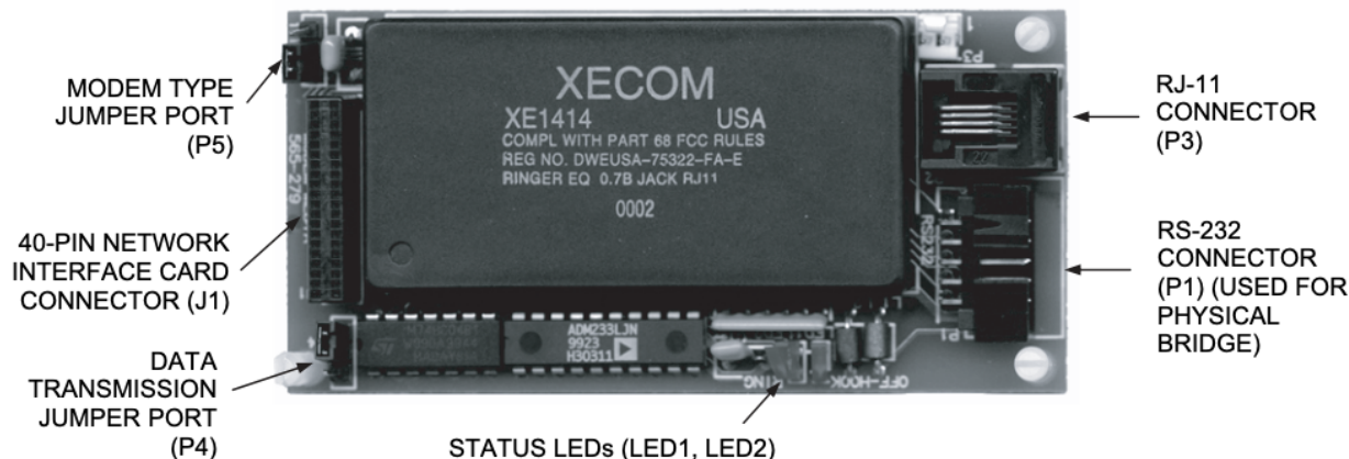
Figure 4-6. The 4100-6055 Modem Media Card (565-279 or 566-338)
