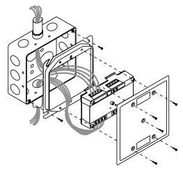
**SIGA-MCC1** and **SIGA-MCC2**: mount the UIO motherboard inside a suitable EDWARDS enclosure with screws and washers provided. Plug the SIGA-MCC1 or SIGA-MCC2 into any available position on the motherboard and secure the module to the motherboard with the captive screws. Wiring connections are made to the terminals on the motherboard (see wiring diagram). UIO motherboard terminals are suited for #12 to #18 AWG (2.5 mm² to 0.75 mm²) wire size.
